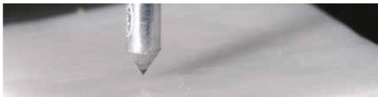
Surface roughness tests
